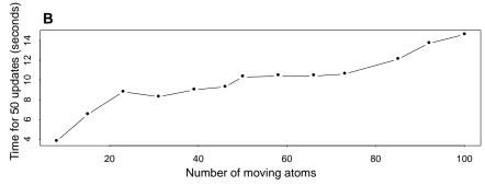
Figure 4: Time for 50 updates of the triangulated SES of the FIV protease during the MD simulation as a function of the number of moving atoms (A) and deleted RS-faces(B).
