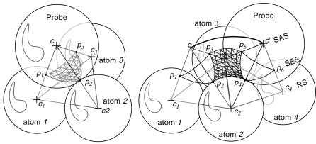
Figure 1: Probe in a fixed position defining an RS-face  $(c_1,c_2,c_3)$ , an SES spherical reentrant face  $(p_1,p_2,p_3)$  and an SAS vertex c.
